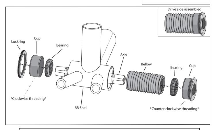
\*\*\*Fully grease both bearings with applicable grease (Not Included) before installing.\*\*\*
