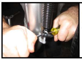
Install spring and use a screwdriver as shown (be careful, screwdriver can be sharp) to insert eyebolt into frame bracket. You will need help to install the nut. Use caution, the spring is very strong.
