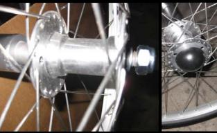
Install rear wheels, with washer behind the axle nut. Note: the axle nuts must NOT be too tight. Their should be up to 1mm of side to side movement of the hub on the axle.
