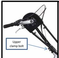
Adjust chain tension by pulling the stem out and tightening the upper clamp bolt.
