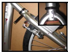
Note that spring bracket goes into UPPER hole in fork.
