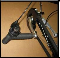
Install and tighten securly the hand pedal assemblies using a standard pedal wrench.
