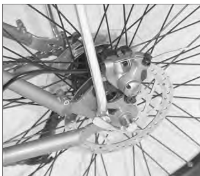
Shimano mechanical disk brakes provided lots of stopping power for the EZ-Tandem after we gave them a tune-up. Plenty of adjustability makes getting comfy on the seats easy to do.
