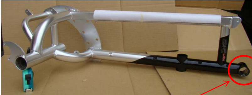
Right Rear 68291 for 30mm O.D. bearing 68599 for 32mm O.D. bearing
